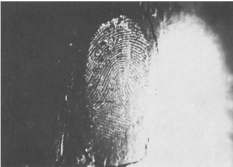
FIG. 2—Latent print on wood vapor stained with 9-methylanthracene following cyanoacrylate fuming and developed under excitation with an UV lamp.
